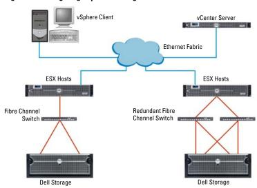
Figure 3. Configuring vSphere 4 Using Dell Fibre Channel SAN
